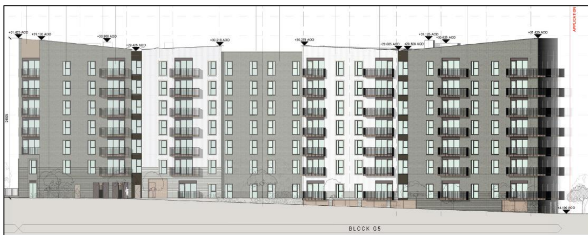
Figure 3: Typical Elevation Glazing to Wall Ratio - Block G5 (East)
